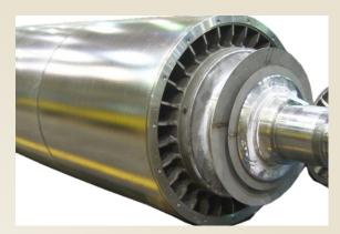
Cambering specification Upto 3mm on Diameter.
